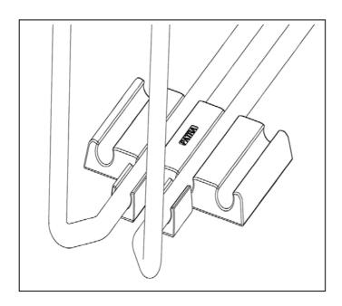
Select spacing and push the chair frame down firmly to locate.
