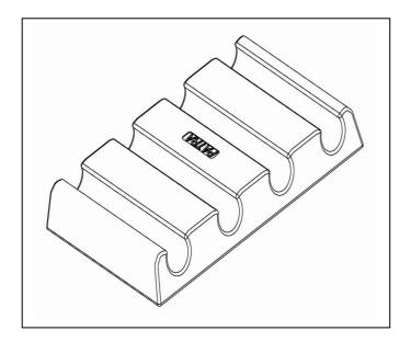
Place the linking "block" on the floor and position chairs over the device.
