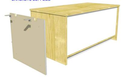
OFFER UP THE INFILL PANEL TO THE END PANEL OF THE DESK, ENSURING AN EVEN BREAK (2mm) FRONT AND BACK. USE THIS INFILL PANEL AS A JIG TO POSITION THE BRACKETS ON THE DESK.
